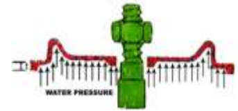
THIN WALLED CORRUGATE SHAPED DIAPHRAGM
