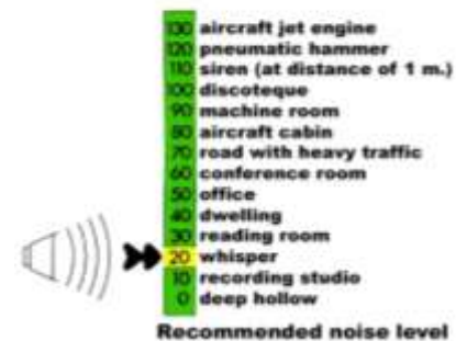
Noise levels of some typical sources with the values in dB
