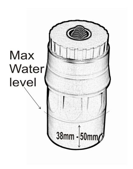
NOTE: there will be a short delay in shut-off the first time the Variflot is used while the control chamber fills with water.
